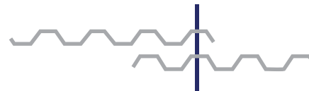
Double position (improves waterproofing)
